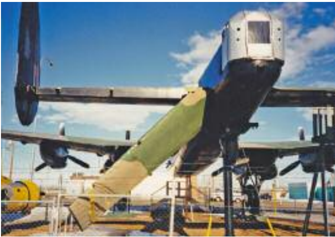
FM159's port elevator after the windstorm. The elevators had been covered with tin after the original fabric was destroyed.
