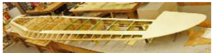
The interior, wooden structure of the Anson's 23 foot wide horizontal stabilizer. It will be covered with plywood and fabric.
