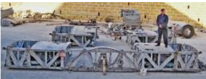
This wing framework, together with numerous other components and engines that have been acquired, is the beginning of the re-building of a Halifax Bomber for the museum.
