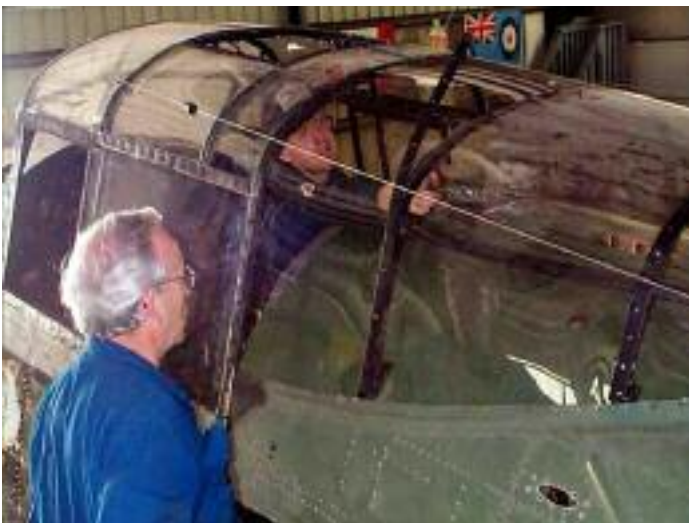
The restoration of FM159's canopy
