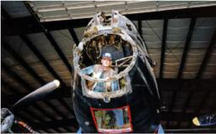
Looking down from the bomb aimer's position, shortly after FM159 had been rolled into the building and the tin covering the broken perspex had been removed.
