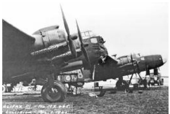
Following a mid-air collision, this Halifax was somehow flown back to base but without the bomb aimer and navigator who were in the nose section
