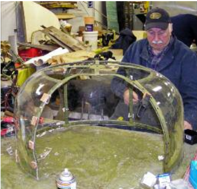
Working on the perspex gun turret dome for the Bristol Blenheim
