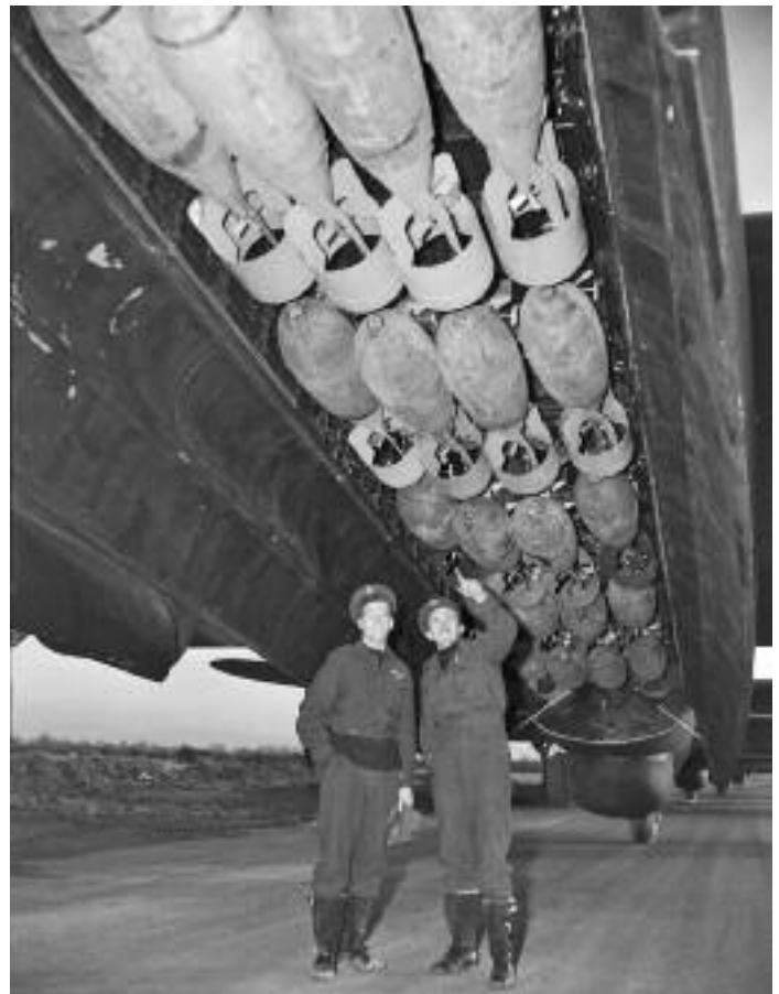
The Lancaster's wing spars were within the fuselage allowing for a huge, unimpeded bomb bay but creating a significant obstacle for the aircrew.
